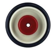
5" x 1 1/4" crown tread polyurethane shopping cart wheel with 5/16" QuadX friction bearing.
