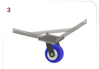
Swivel plate bolts or welds to angle iron frame and corner brace.
