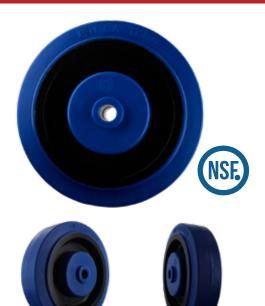
P&H's metric products include this premium material handling wheel that performs exceptionally well for operations such as conveyor tow lines where wheels run continuously. These wheels combine the load bearing qualities found in steel with an exceptional level of resistance to most chemicals, high tensile strength, low rolling resistance and non-marking tread. Stronger than polypropylene, these wheels have an excellent level of resilience.
