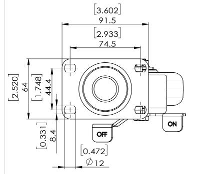
Durometer: Shore D90 (+/-5) Wheel P/N: 35-171M-B
